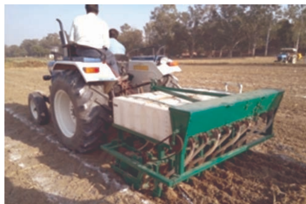
Wheat sowing with developed UAN Applicator
