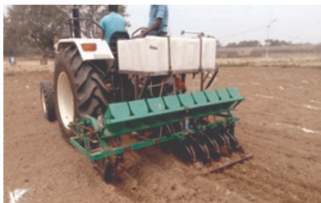
Retrofitted UAN applicator on direct paddy seeder
