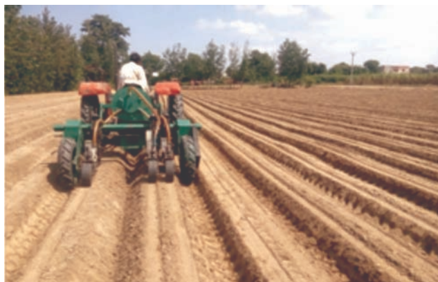
Testing of pneumatic precision planter on raised bed
