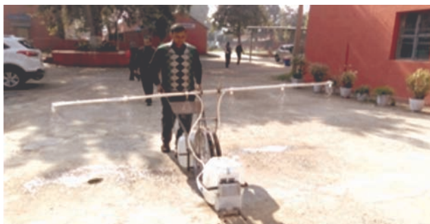
Testing of walking type battery operated boom sprayer
