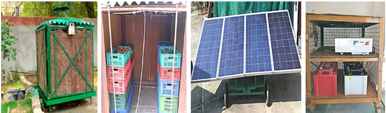
Solar powered evaporatively cooled storage structure with solar power pack
