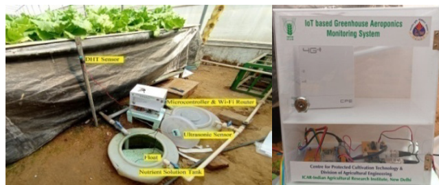
IoT based Greenhouse Aeronics Monitoring System
